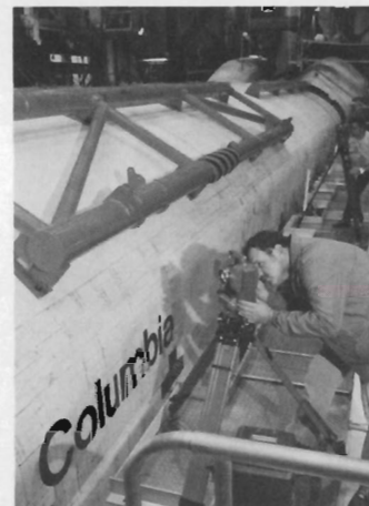
Before the space shuttle Columbia's 1982 flights, engineers used an HP 3822A coordinate determination system to align component parts. The Loveland-built instrument checked the position of the payload in the cargo bay and the alignment of door hinges and booster rockets.
