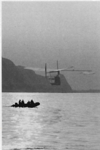
It took pilot Bryan Allen two hours and 49 minutes to pedal the Gossamer Albatross across the English Channel in June 1979. An HP 9820 desktop computer, linked to an HP 9862A plotter, was used to design the airfoil used in the wings and propellers of the 75-pound, 96-foot wide aircraft.
